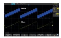
Enhanced Resolution (Eres) mode can improve the SNR without needing a repetitive waveform. Extra resolution bits can be added 0.5 bits at a time up to +3 bits.
