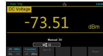
The dB and dBm functions allow relative measurements to either a stored relative value or 1 milliwatt depending on which function is chosen.
