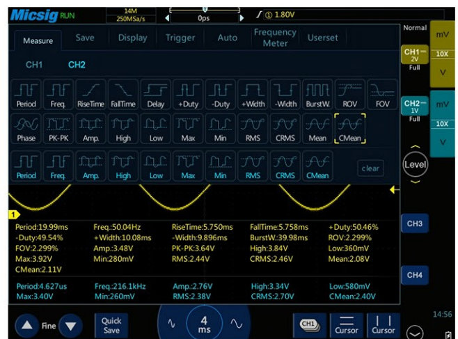
31 automatic measurements. Various automatic measurements can meet different frequency measurement demand. It can be display all in one page.
