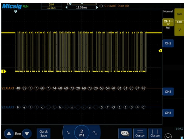
Support serial triggering and decode (I2C, SPI, RS232/UART,CAN, LIN) and Aerospace and defence (MIL-STD 1553, ARINC 429). Two formats to display decoding, text and graphic.
