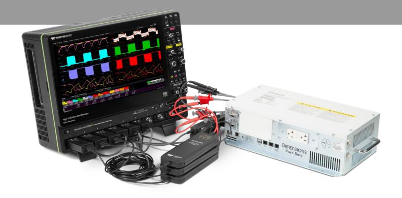
WaveRunner 8000HD 12-bit oscilloscopes deliver 8 analog channels (16 with OscilloSYNC), 3-phase power analysis software, and high performance probes for inverter subsection, power system and control testing.
