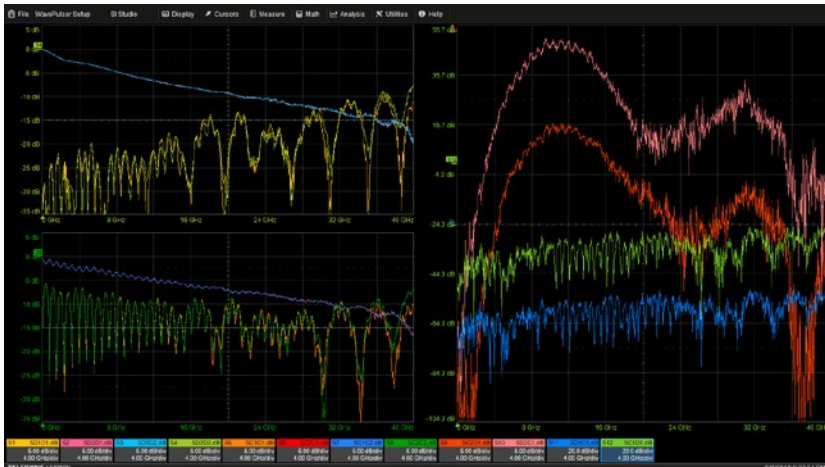
Mixed-mode return and insertion losses are simultaneously displayed.
