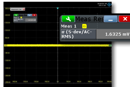
The RTO2000's 8-bit ADCs and higher noise mean lower signal fidelity.
